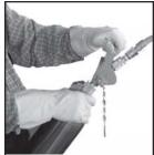
14. Stop the filling process by first closing the X-10C valve so the safety snap device is engaged. Press in the safety pin (hanging from the chain) before proceeding.
