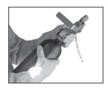
to bend the drawtube, as chemical pickup from the bottle will be affected. You can check the drawtube bend by comparing the tube to the illustration on the next page.
